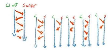
Each of those pipes still incurs the limitation of synchronous request/response pairs. If a web page has more than 6 additional resources that need to be loaded (typical modern sites can have 40+), then the browser will still be waiting a significant amount of time for round-trip latency on each of these pipes.
